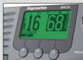
Dual Channel Display (2UP Mode) displays active channel and standby channel simultaneously
