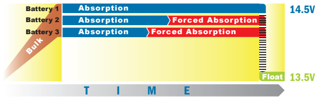
Example of Flooded Lead Acid Battery
