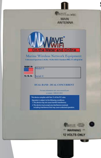
The EC ER DB comes with 25ft of low loss cable that is then connected to a powerful Dual Band Omni-Directional antenna giving the system an incredible amount of range. The system is a more affordable midrange solution when comparing our most powerful EC HP DB and shorter range Rogue systems.
