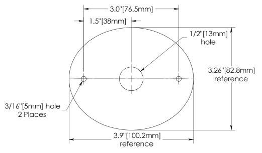
3. Feed all of the Control Panel wires through the center hole of the small gasket, then place the gasket underneath the control through the two threaded mounts.
