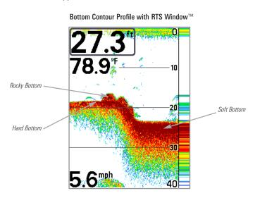
The sonar returns from the bottom, structure, and fish can be represented as **WhiteLine™** or **Structure ID®**. See *Sonar Menu Tab: Bottom View* to set the bottom view.
