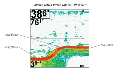
The sonar returns from the bottom, structure, and fish can be represented as either **WhiteLine**<sup>TM</sup> or **Structure ID**<sup>®</sup>. See *Sonar Menu Tab: Bottom View* for details on how to set the bottom view.
