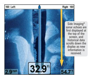
The main benefit of Side Imaging® sonar to anglers is that it provides an overall survey of a large area of water. This gives you a better understanding of the bottom topography and how structure is oriented for more efficient fishing.
