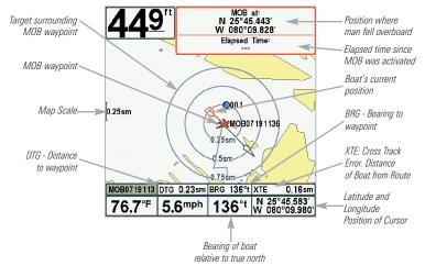
Cancel MOB navigation: From the Navigation X-Press<sup>™</sup> Menu, select Cancel MOB, and press the RIGHT Cursor key. Canceling MOB navigation removes the route and any waypoints created using the GOTO key but does not remove any saved routes from memory.
