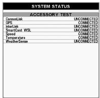
**Accessory Test** lists the accessories connected to the system.
