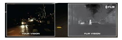
The above images show a comparison of typical night time driving compared to using the Helios thermal imager. The image on the left is from an ordinary digital camera and shows the amount of visible light as illuminated by oncoming headlights. The image on the right is a thermal image created by the Helios thermal imaging camera. Note the Helios camera is sensitive to warm objects, such as the people, and provides visibility over a much greater distance.
