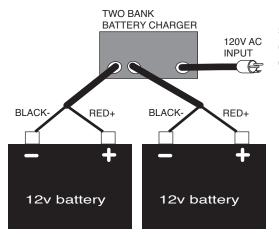
NOTE: If batteries are connected in series for 12/24 - 24V, the series connection wire can be left in place during charging.
