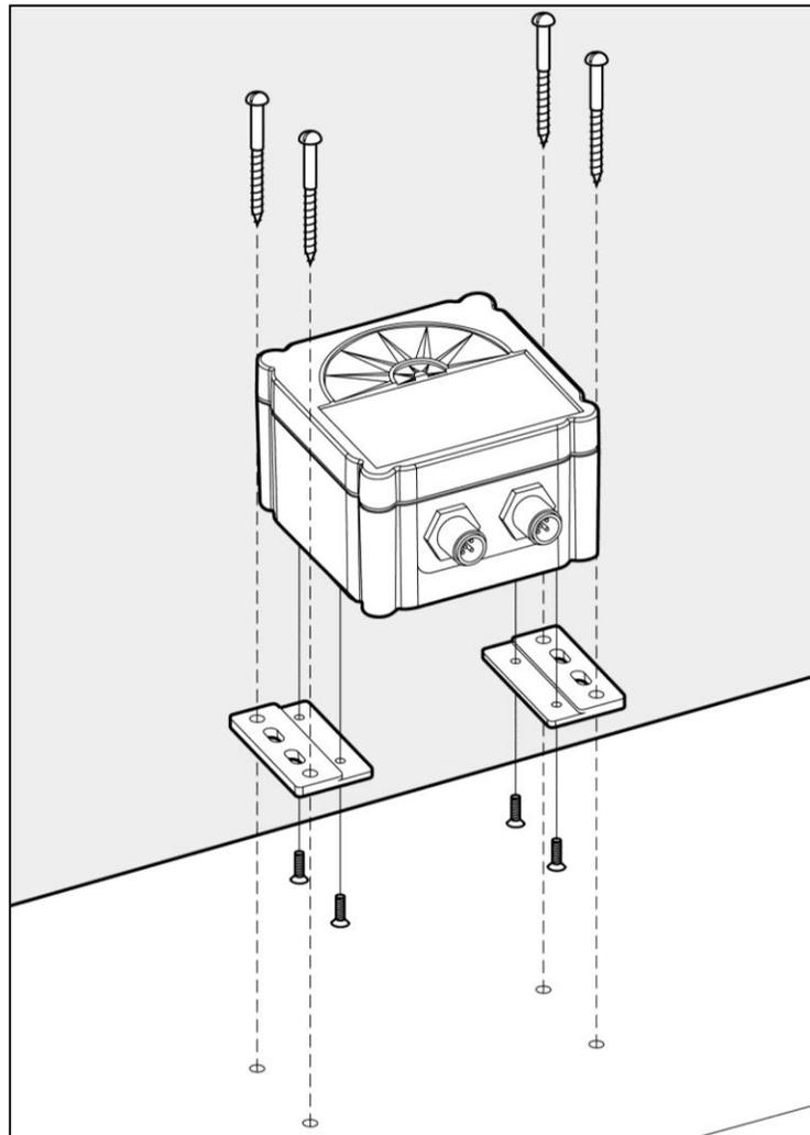
**Figure 1 – Mounting the SSC300 to a Horizontal Surface**
