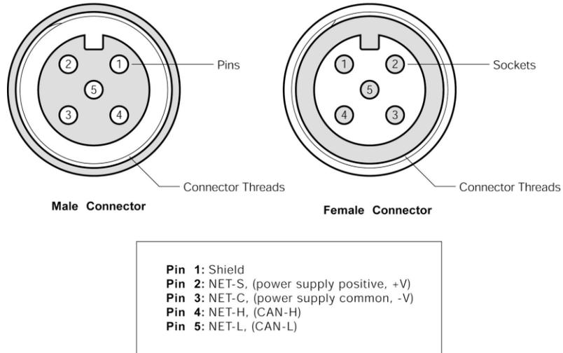
**Figure 4 – NMEA 2000®/Power Connector Face Views**
