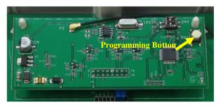
If the remote FOB must be replaced, the new one can easily be coded to the wireless receiver. To do this, power the PD Box on, then press the programming button on the receiver and release. Then press and release the MODE button on the wireless receiver, repeat this until the code is picked up by the receiver. This can be verified by seeing the Shadow-Caster Lights changing color. Note that the wireless controller will only support one remote at a time.
