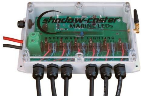
SCM-PD shown with optional wireless Controller Installed.
