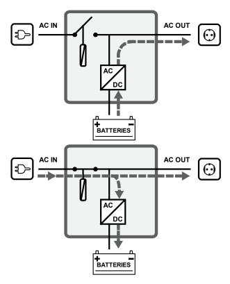
Power sharing mode: The CombiMaster automatically reduces its battery charger output when the load connected to AC
