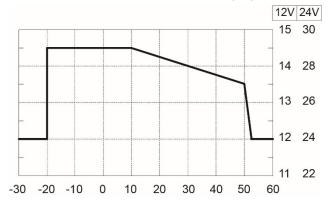
Figure 7: Temperature compensated charging
