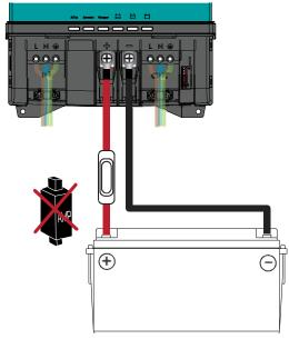
**Step 9.** Attach the battery temperature sensor to the casing of the battery bank. Then plug the temperature sensor cable into the "temp.sensor" jack.
