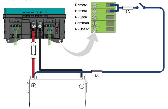
• Use both contacts to connect an external switch. In this case, the CombiMaster's main switch must be in the on position (I). Closed = On, Open = Charge only.
