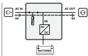
Load on AC OUT ≥ AC IN Limit
