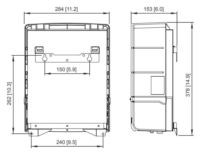
Figure 9: Dimensions 12V/2000VA-60A and 24V/2000VA-40A in mm [inches]
