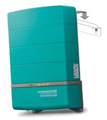
**Step 4.** Fix the CombiMaster to the surface by fastening two screws at the lower side of the case as well.
