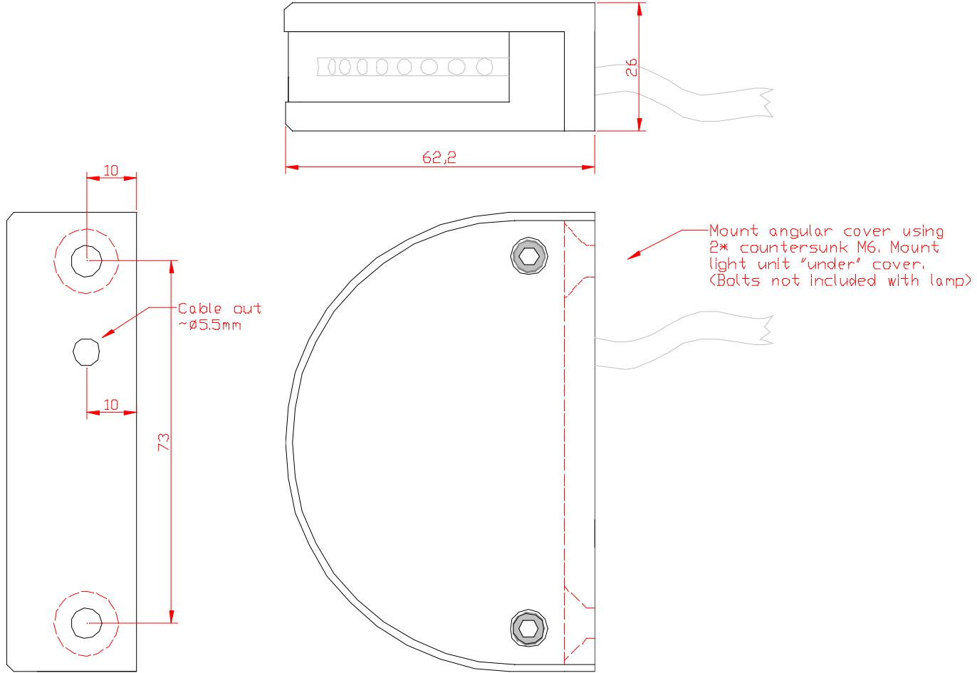
**To mount the light use the supplied grey thick plastic piece.**
