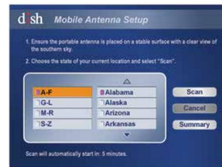
If the *Mobile Antenna Setup* screen does not display, press **MENU, 6, 1, 1** on your DISH remote.
