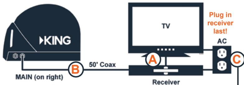
**Do not over tighten coax connections! Do not pull on coax.**
